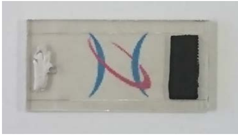
Figure 5. transparent nano-particle solar cell
